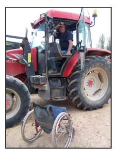
The tractor only needed modifications to the brake as it has a clutch on the gear lever and the steering column and therefore did not require modifications.
