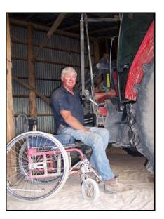
To access the tractor cabin, Wayne transfers into the seat affixed to the winch pole, he then winds the winch to the appropriate height and transfers to the trainee seat, then to the driver's seat. He swings the seat out of the way, secures the seat and closes the door.
