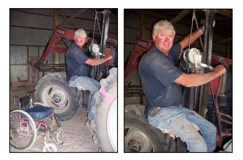
This tractor is a manual so Wayne has put a lever to pull down the clutch and brake with a locking mechanism to hold the clutch down. This enables him to change gears with the same arm as they are both on the same side of the tractor.
