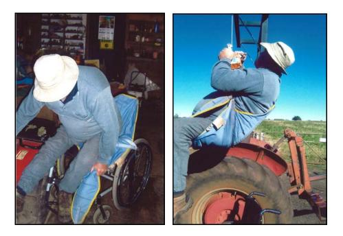
He transfers from his quad onto the sling placed on the seat of his wheel chair and clips himself to the winch attached to the gantry frame, which extends outside the line of the rear tyre. He then winches himself up to above the height of the mud guard of the tractor; once at the correct height he slides along the gantry to above the tractor seat and lowers himself down into position and drives away.
