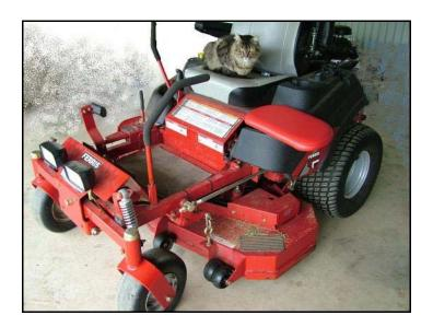
The Ferris Zero Turn mower required very little modification. A seat was made with a steel frame, covered in foam and vinyl, which slid onto the base which held the left control arm. That control arm was then placed onto a supporting steel peg at the front left of the machine to help Sam support himself as he transferred onto the temporary seat, then across onto the bucket seat. He then removes the temporary seat, putting the control arm back in place to mow.
