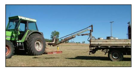
The big challenge was keeping the seat level as the hoist went up and down. They devised a see-saw mechanism above the hoist to solve this problem. The hydraulics of the hoist were wired to a remote control panel which moves the seat up or down.
