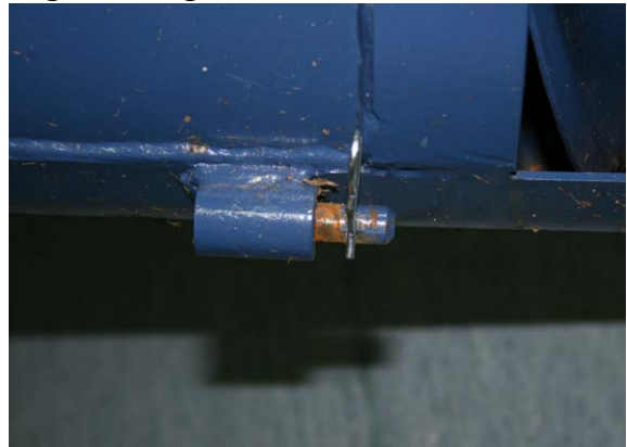
Detail of lug and pin to attach outer guard
