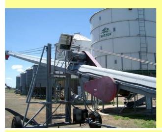
Ensure that all auger flights, engine pulleys, drive belts and shafts are properly guarded and that the guards are in good condition before using all augers.
