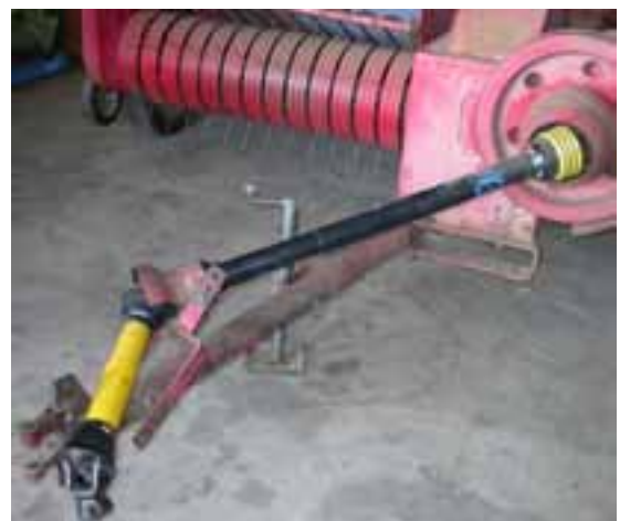
Figure 4.4: PTO transmission system for a rectangular hay baler.
