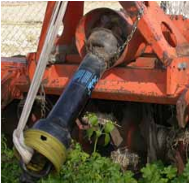
Figure 1.1 Clip-held removable Master Guard covering the connection of PTO shaft to tractor PTO.
