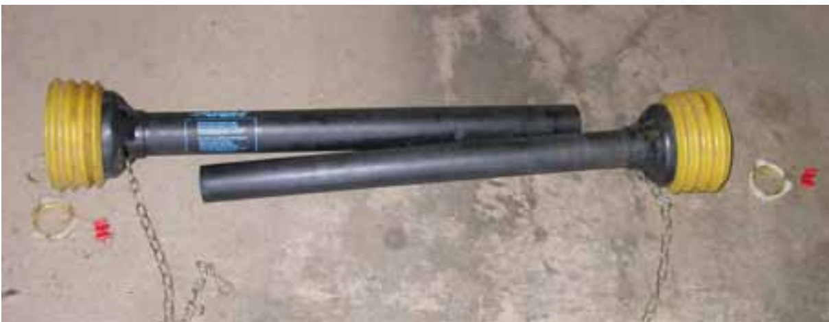
Figure 1.3: Generic PTO shield composed of : two telescoping black poly pipes or tubes, yellow bellows-like cones at each end, white nylon expandable bearings that clip into a groove on each end of the shaft, red plastic locking clips that lock the guard to the bearing, and restraining chains to stop the guard from rotating.
