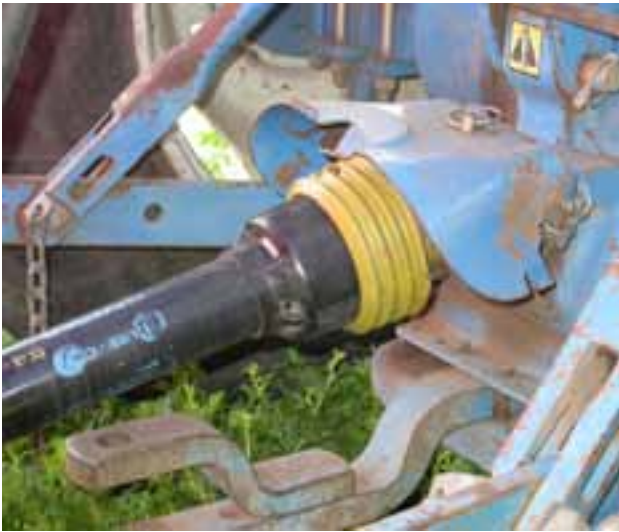
Figure 1.1 Clip-held removable Master Guard covering the connection of PTO shaft to tractor PTO.
