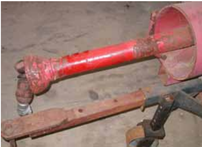
Figure 4.2: Steel PTO guard. Note resting hook to support PTO when not in use, and avoid damage by dropping onto the drawbar below.
