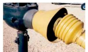
A different model posthole digger. The same problem of exposed universal joint is evident.
