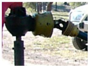
**Power-take-off shaft universal joint exposed when digger is starting to dig.** Photograph courtesy R Houghton
