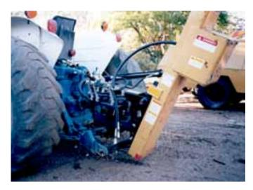
Three-point-linkage mounted post driver.
