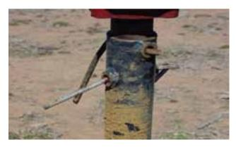
Picture showing shear pins replaced with steel rods. The protruding ends make this very dangerous.
