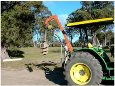
Linkage mounted posthole digger Photograph courtesy R Houghton
