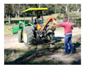
The worker standing behind the digger is in danger of being struck and/or entangled if the auger hits an object and jumps from the hole. Wire, steel posts and tools lying near the posthole increase the hazard. Photograph courtesy R Houghton
