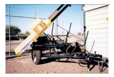
Trailer mounted post driver. Operation is hydraulic, operating from the tractor remote hydraulic lines.
