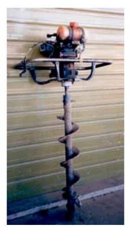
Portable engine-driven posthole digger
